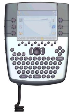
TOUR ONLINE uses data transmitted from palm computers (see an example above) that are connected to the black-box of the tanker trucks, linked via GPS/GPRS to the base station
